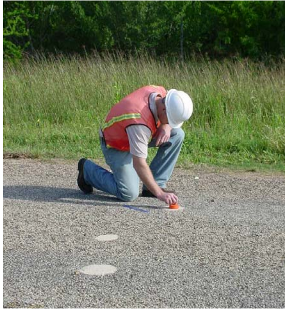
Figure 15: Researcher performing Sand Circle Test
