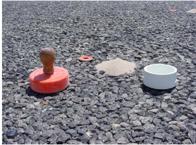
Figure 14: Testing Equipment (hockey puck, washer, sieved sand, PVC cup)
